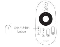
2. Short press "n" button 3 times within 3 seconds when light on.
