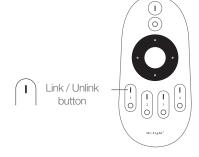
2. Short press "\" button 5 times within 3 seconds when light on.
